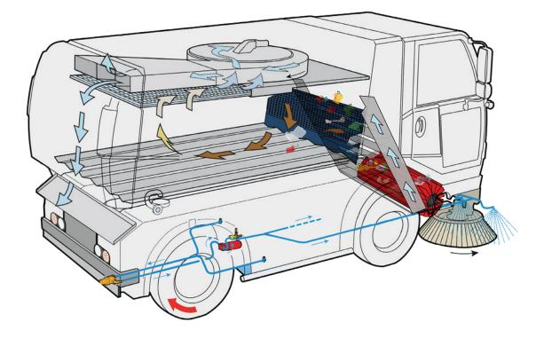
**The combined mechanical / suction / filtering** collection guarantees powerful and fast loading of any type of material from dust to leaves, as well as gravels ad large debris. An effective suction system optimises the collection of dust and light materials and the filtering system, made up of a battery of polyester filters, captures fine dust particles up to PM 2.5 under all operating conditions, by eliminating almost completely the introduction of pollutants into the atmosphere.
